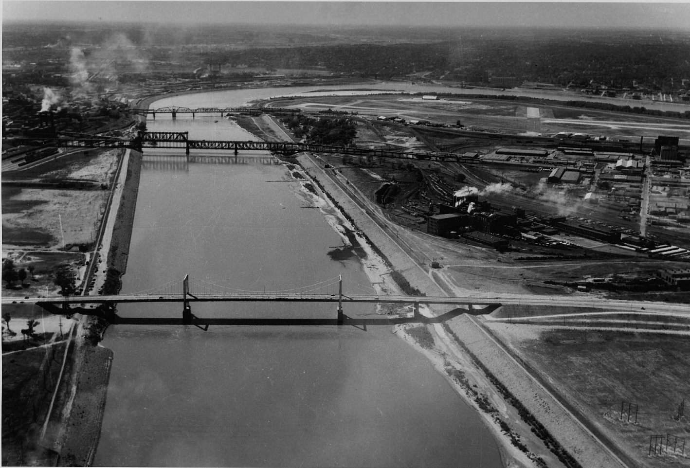
MISSOURI RIVER IMPROVEMENT CHANNEL STABILIZATION AND NAVIGATION PROJECT KANSAS CITY DISTRICT AERIAL VIEW WEST (UPSTREAM) FROM APPROXIMATE RIVER MILE 376, SHOWING PORTION OF RIVER FROM KANSAS CITY REACH TO KANSAS RIVER BEND. LEVEE AND BANK PROTECTION ALONG LEFT BANK IN NORTH KANSAS CITY UNIT, LEVEE AND BANK PROTECTION ON RIGHT BANK IN EAST BOTTOMS UNIT. BRIDGES FROM BOTTOM UP ARE: NEW PASEO BRIDGE; (A.S.B.) HIGHWAY & RAILWAY BRIDGE AND E.B. & Q. R.R. (HANNIBAL) RAILWAY AND HIGHWAY BRIDGE. CONFLUENCE OF KANSAS AND MISSOURI RIVERS IN CENTER BACKGROUND. 23 SEPTEMBER 1954
